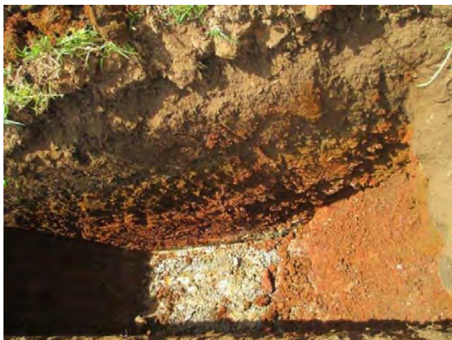
Residual clay soil profile characteristic of the site and broader area
